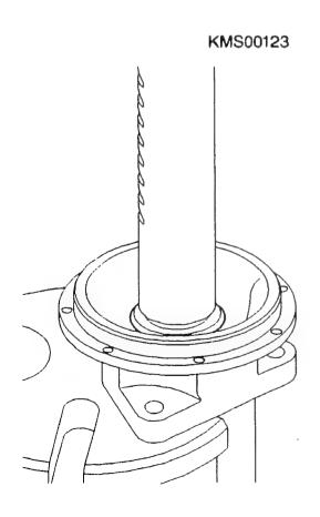
Checking intermediate bearing
